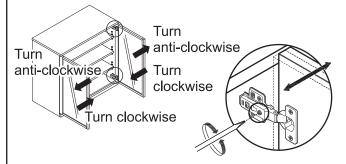
\* There are two hinges on each door. Alternately turn the screws clockwise or anti-clockwise to make adjustments.
