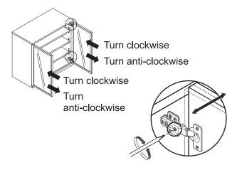
\* There are two hinges on each door. Alternately turn the screws clockwise or anti-clockwise to make adjustments.
