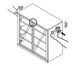
1 Find the position where the doors become aligned by tilting the main unit a little at a time to the left or right.
