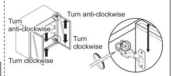
There are two hinges on each door. Alternately turn the screws clockwise or anti-clockwise to make adjustments.
