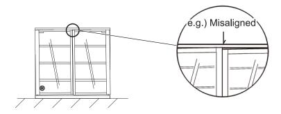
If the doors are misaligned, gently push the side boards of the main unit with hands. If this does not correct the misalignment, go to steps ① to ③ below.
